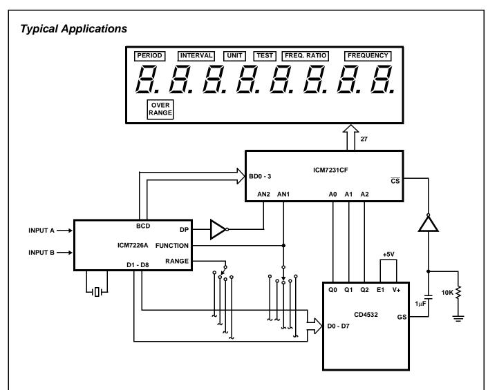
NOTE: The annunciators show function and the decimal points indicate the range of the current operation. the system can be efficiently battery operated.
