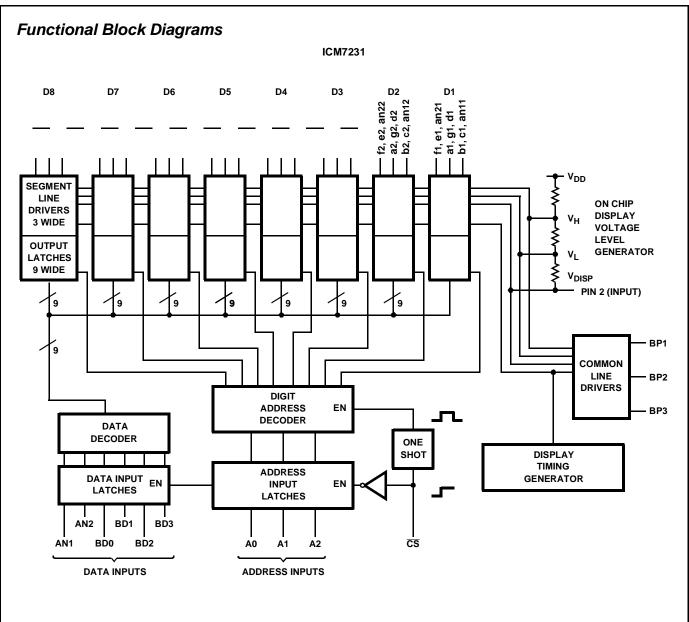
NOTE: See Figure 13 for display segment connections.
