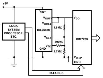
FIGURE 12. FLEXIBLE TEMPERATURE COMPENSATION
