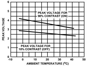
FIGURE 9. TEMPERATURE DEPENDENCE OF LC THRESHOLD
