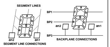
FIGURE 4. CONNECTION DIAGRAMS FOR TYPICAL 7-SEGMENT DISPLAYS
