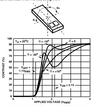
FIGURE 8. CONTRAST vs APPLIED RMS VOLTAGE
