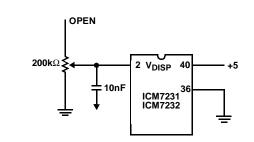
FIGURE 10. SIMPLE DISPLAY VOLTAGE ADJUSTMENT
