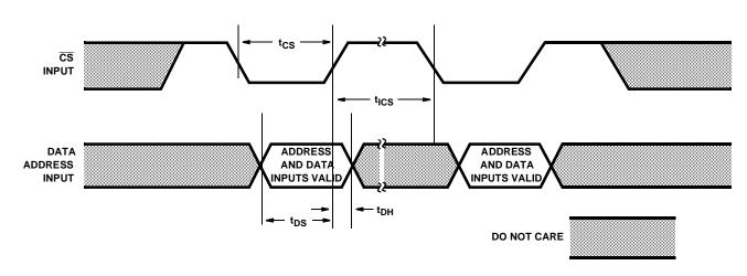
FIGURE 1. ICM7231 INPUT TIMING DIAGRAM
