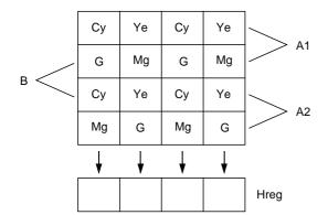
As shown in the left figure, fields are read out. The charge is mixed by pairs such as A1 and A2 in the A field. (pairs such as B in the B field)
