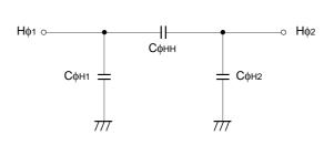
Vertical transfer clock equivalent circuit
