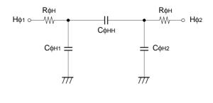
Vertical transfer clock equivalent circuit
