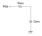
Reset gate clock equivalent circuit
