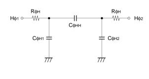
Vertical transfer clock equivalent circuit
