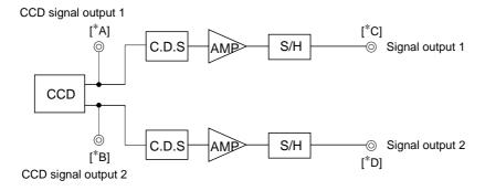
Note) Adjust the amplifier gain so that the gain between [\*A] and [\*C], and between [\*B] and [\*D] equals 1.
