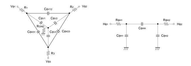
Vertical transfer clock equivalent circuit
