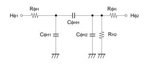
Vertical transfer clock equivalent circuit
