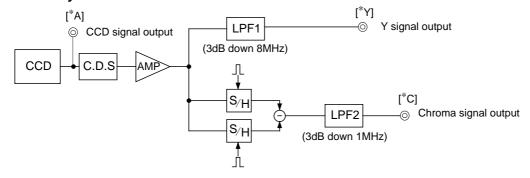
**Note)** Adjust the amplifier gain so that the gain between [\*A] and [\*Y], and between [\*A] and [\*C] equals 1.
