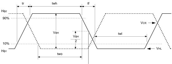
Cross-point voltage for the H $\phi$ 1 rising side of the horizontal transfer clocks H $\phi$ 1 and H $\phi$ 2 waveforms is Vcr. The overlap period for twh and twl of horizontal transfer clocks H $\phi$ 1 and H $\phi$ 2 is two.
