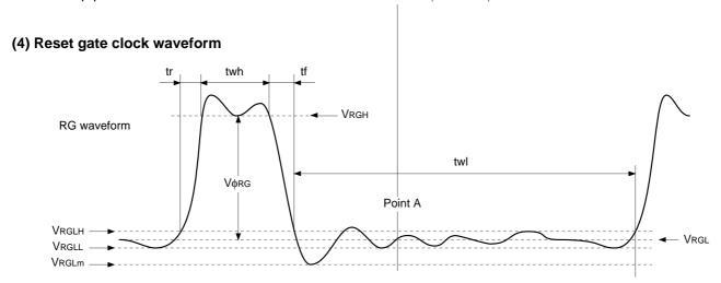
VRGLH is the maximum value and VRGLL is the minimum value of the coupling waveform during the period from Point A in the above diagram until the rising edge of RG. In addition, VRGL is the average value of VRGLH and VRGLL.
