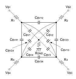
Vertical transfer clock equivalent circuit
