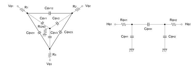
Vertical transfer clock equivalent circuit
