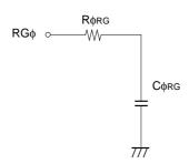
Reset gate clock equivalent circuit
