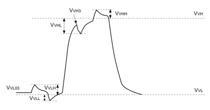
$V_{VH} = V_{VH02}$  $V_{VL} = (V_{VL01} + V_{VL03})/2$   $V\phi$ V1 = VVH1 - VVL01  $V\phi$ V2 = VVH02 - VVL2  $V\phi$ V3 = VVH3 - VVL03
