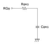
Reset gate clock equivalent circuit
