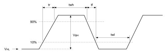
(4) Reset gate clock waveform
