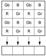
The primary color filters of this image sensor are arranged in the layout shown in the figure on the left (Bayer arrangement).
