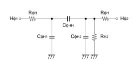
Vertical transfer clock equivalent circuit
