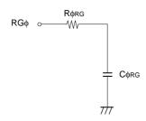
Reset gate clock equivalent circuit
