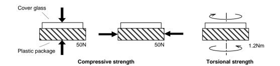
b) If a load is applied to the entire surface by a hard component, bending stress may be generated and the package may fracture, etc., depending on the flatness of the bottom of the package. Therefore, for installation, use either an elastic load, such as a spring plate, or an adhesive.
