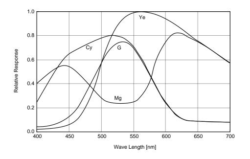
**Spectral Sensitivity Characteristics** (excludes both lens characteristics and light source characteristics)
