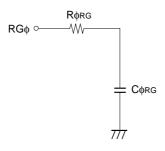
Reset gate clock equivalent circuit
