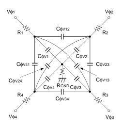
Vertical transfer clock equivalent circuit
