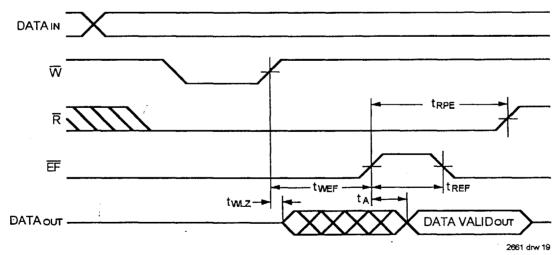
Figure 17. Read Data Flow-Through Mode
