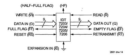
Figure 12. Block Diagram of 2048 x 9/4096 x 9/8192 x 9/16384 x 9 FIFO Used in Single Device Mode
