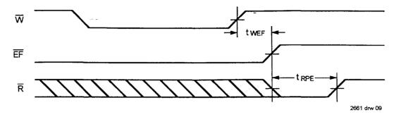
Figure 7. Minimum Timing for an Empty Flag Coincident Read Pulse.
