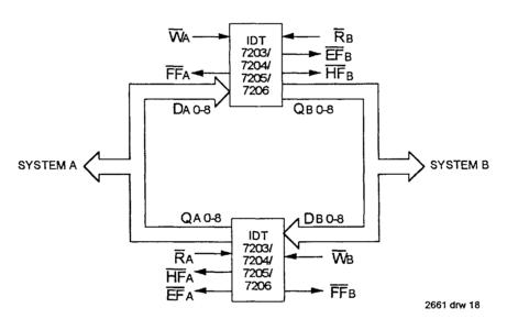
Figure 16. Bidirectional FIFO Operation
