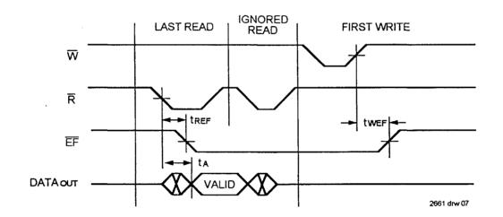
Figure 5. Empty Flag Timing From Last Read to First Write
