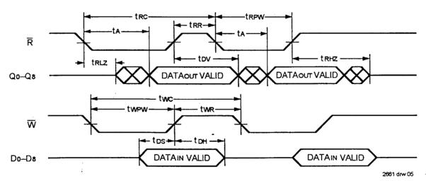
Figure 3. Asynchronous Write and Read Operation
