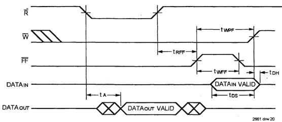
Figure 18. Write Data Flow-Through Mode
