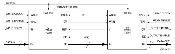
Figure 22. Block Diagram of 131,072 x 9 and 262,144 x 9 Depth Expansion
