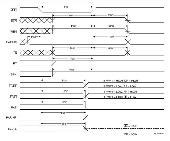
Figure 5. Master Reset Timing
