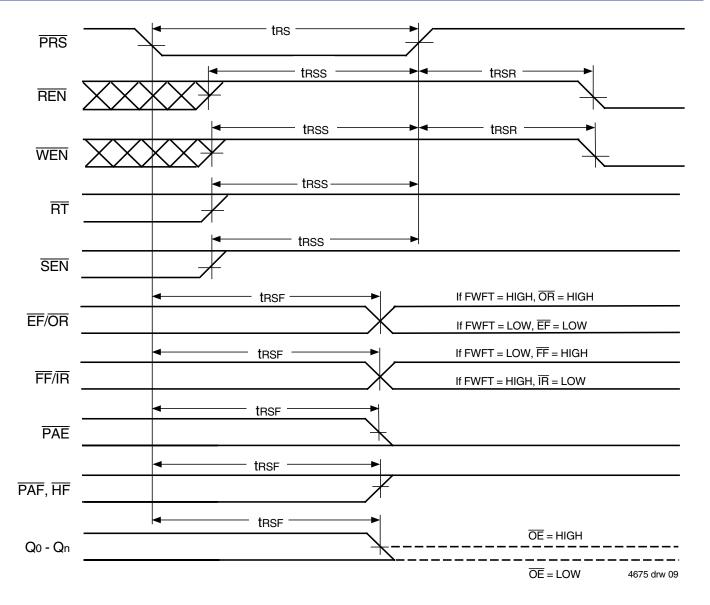
Figure 6. Partial Reset Timing
