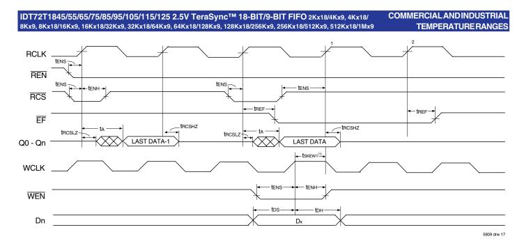
1. tskew1 is the minimum time between a rising WCLK edge and a rising RCLK edge to guarantee that  $\overline{\text{EF}}$  will go HIGH (after one RCLK cycle plus tree). If the time between the rising edge of WCLK and the rising edge of RCLK is less than tskew1, then  $\overline{\text{EF}}$  deassertion may be delayed one extra RCLK cycle.
