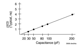
Figure 2b. Lumped Capacitive Load, Typical Derating
