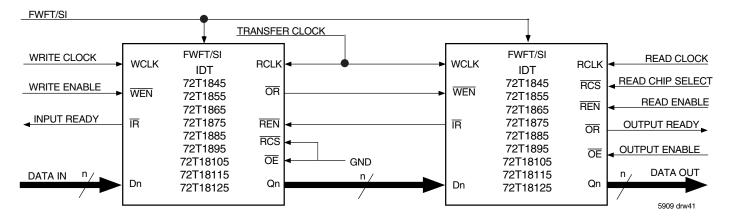
Figure 37. Block Diagram of Depth Expansion For the x18 Input or x18 Output bus Width: 4,096 x 18, 8,192 x 18, 16,384 x 18, 32,768 x 18, 65,536 x 18, 131,072 x 18, 262,144 x 18, 524,288 x 18 and 1,048,576 x 18 For both x9 Input and x9 Output bus Widths: 8,192 x 9, 16,384 x 9, 32,768 x 9, 65,536 x 9, 131,072 x 9, 262,144 x 9, 524,288 x 9, 1,048,576 x 9 and 2,097,152 x 9
