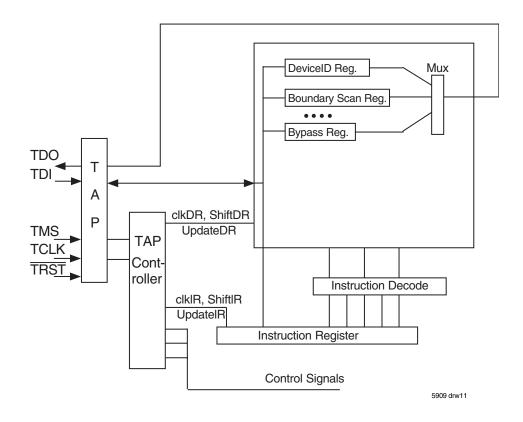
Figure 7. Boundary Scan Architecture
