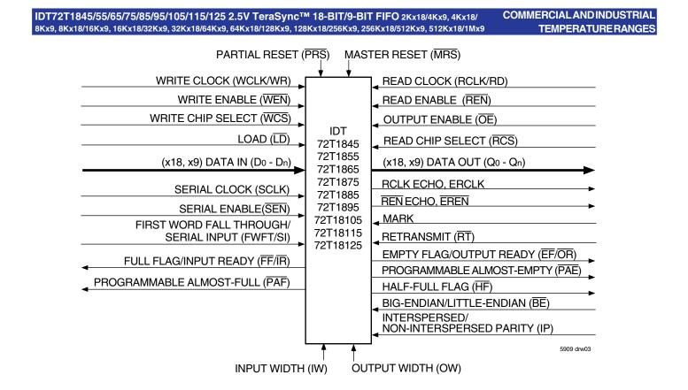
Figure 1. Single Device Configuration Signal Flow Diagram
