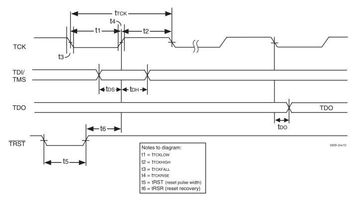
Figure 6. Standard JTAG Timing
