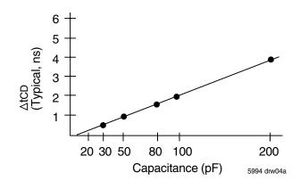
Figure 2b. Lumped Capacitive Load, Typical Derating
