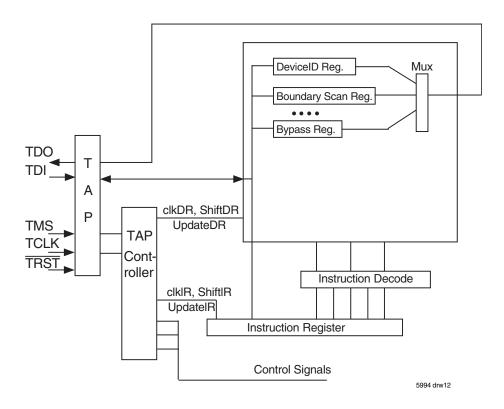
Figure 7. Boundary Scan Architecture
