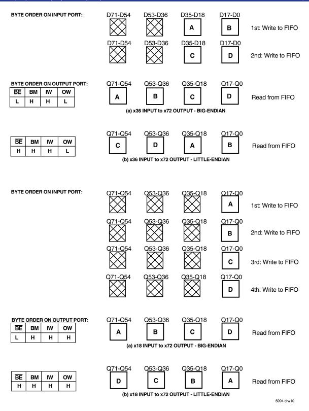
Figure 5. Bus-Matching Byte Arrangement (Continued)
