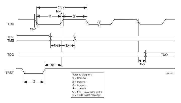
Figure 6. Standard JTAG Timing
