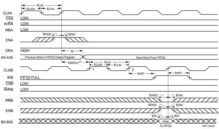
Figure 21. IRB Flag Timing and First Available Write when FIFO2 is Full (FWFT Mode)
