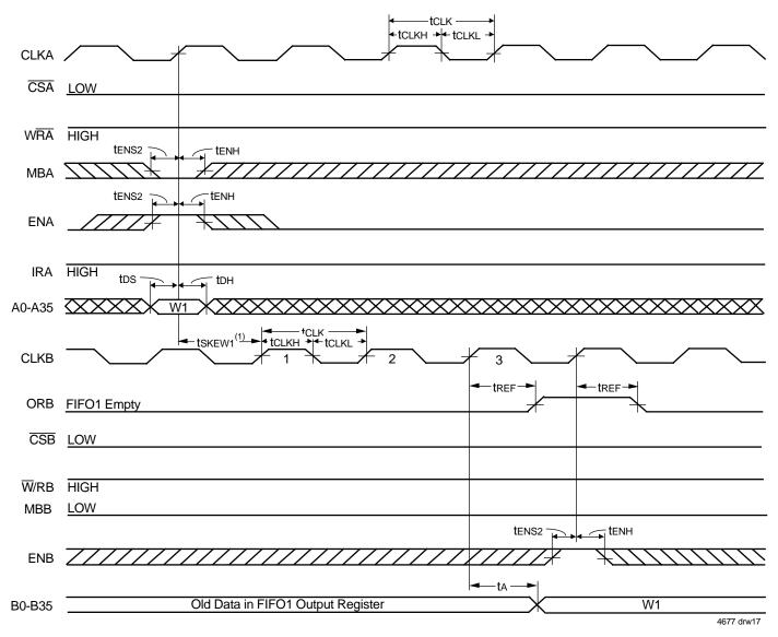
Figure 15. ORB Flag Timing and First Data Word Fall Through when FIFO1 is Empty (FWFT Mode)
