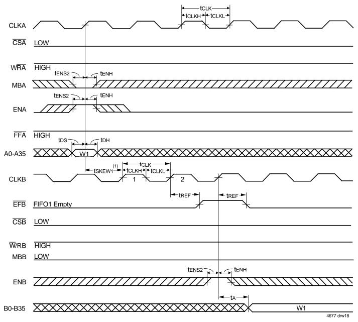
Figure 16. EFB Flag Timing and First Data Read Fall Through when FIFO1 is Empty (IDT Standard Mode)
