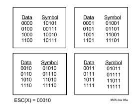
This encode/decode implementation has several very desirable properties. Among them is the fact that the output data bits can be represented by a set of relatively simple symbols;
