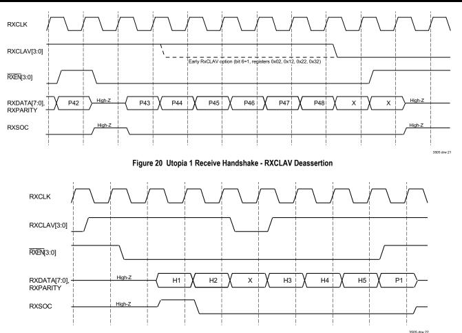
Figure 21 Utopia 1 Receive Handshake - RXCLAV Suspended Transfer (Byte Mode Only) Control and Status Interface
