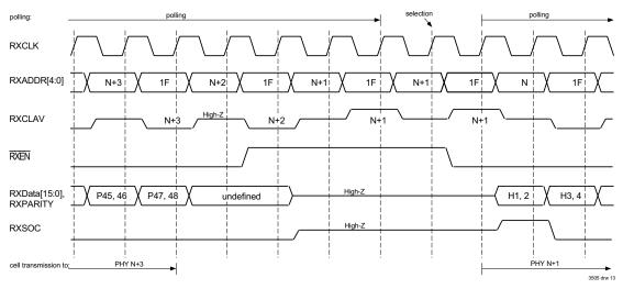
Figure 13 Utopia 2 Receive Handshake - Delay Between Cells
