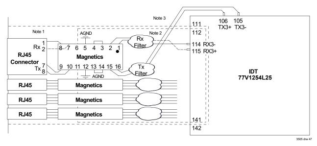
Figure 47 PC Board Layout for ATM Network
