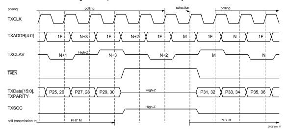
Figure 11 Utopia 2 Transmit Handshake - Transmission Suspended
