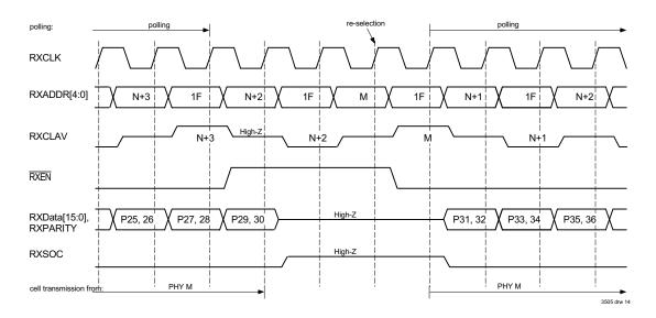
Figure 14 Utopia 2 Receive Handshake - Suspended Transfer of Data
