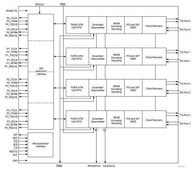
Figure 3 Block Diagram for DPI configuration (MODE[1:0] = 10)
