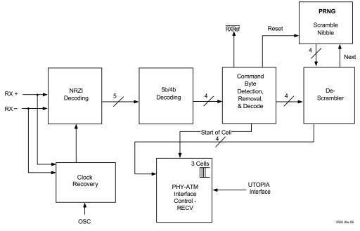
Figure 5 TC Receive Block Diagram
