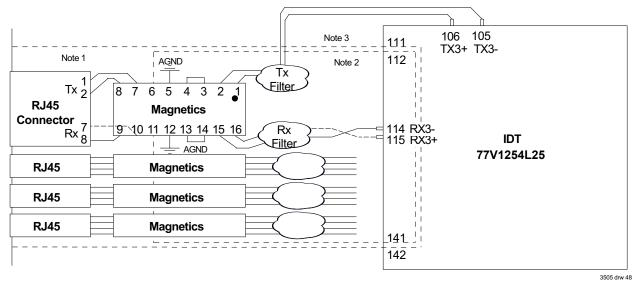
Figure 48 PC Board Layout for ATM User
