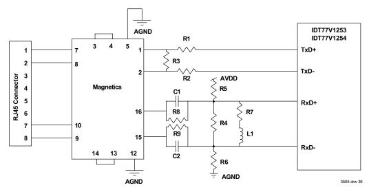
Figure 36 Recommended Connection to Magnetics
