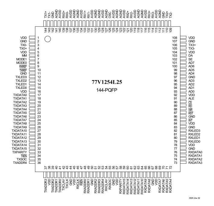
Figure 1 Pin Assignments
