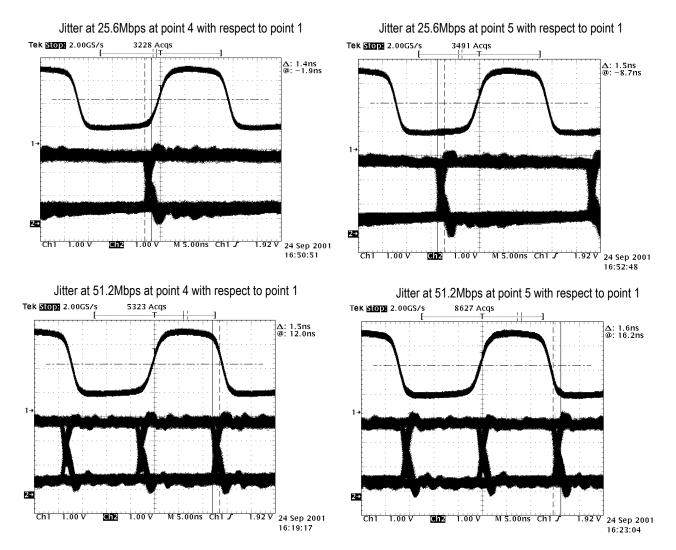
From the above measurements taken, the amount of jitter being added at each TX point is not significant. These tests were also run for extended periods of time (64 hours) and no bit errors were seen.
