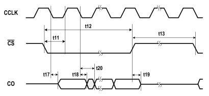
Figure - 10 MPI Output Timing
