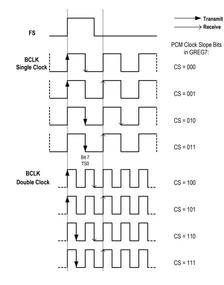
Figure - 3 Sampling Edge Selection Waveform
