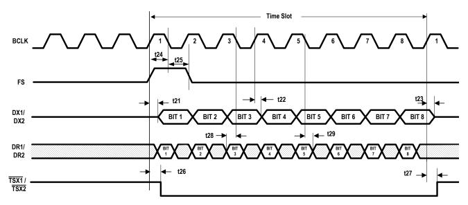
Note: This timing diagram only applies to the situation of receiving data on falling edges and transmitting data on rising edges.
