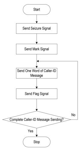
Figure - 6 General Procedure of Sending Caller-ID Signal
