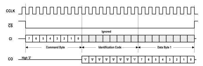
Figure - 2 An Example of the MPI Interface Read Operation (ID = 81H)
