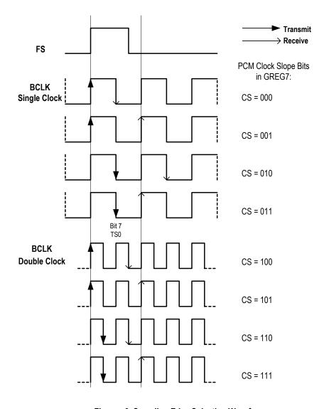
Figure - 3 Sampling Edge Selection Waveform
