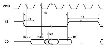
Figure - 8 MPI Output Timing
