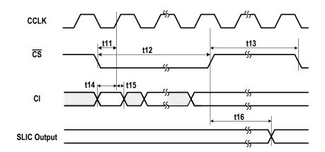
Figure - 7 MPI Input Timing
