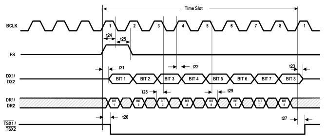
Note: This timing diagram only applies to the situation of receiving data on falling edges and transmitting data on rising edges.
