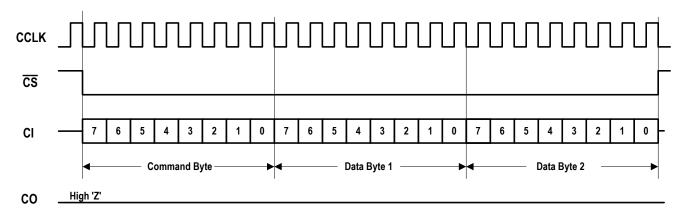
Figure - 1 An Example of the MPI Interface Write Operation
