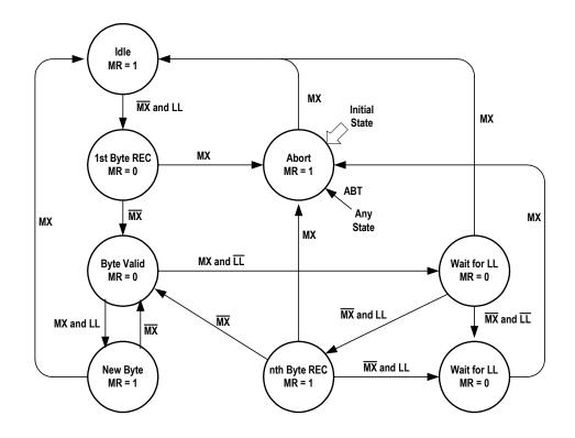
MR: MR bit calculated and transmitted on DU MX: MX bit received data downstream (DD) LL: Last look of monitor byte received on DD ABT: Abort indication to internal source
