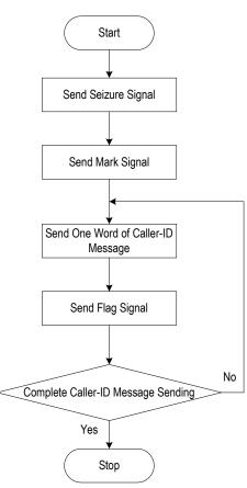
Figure 11 General Procedure of Sending Caller-ID Signal
