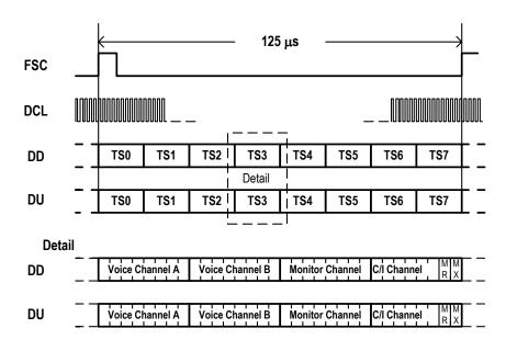
Figure 4 Compressed GCI Frame Structure
