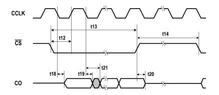
Figure 15 MPI Output Timing
