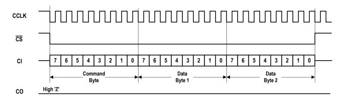
Figure 1 An Example of Serial Interface Write Mode
