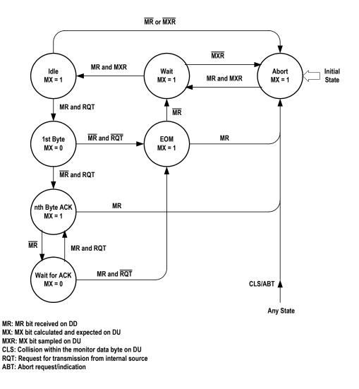
Figure 7 State Diagram of the Monitor Transmitter
