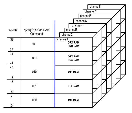
Figure 18 Coe-RAM Address Mapping
