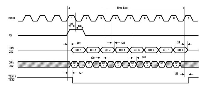
Figure 16 PCM Interface Timing
