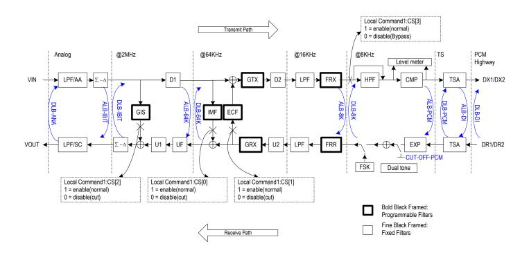
These loopbacks and receive PCM cutoff are controlled by Global Command 26, Local Command 1 and Local Command 2 as shown in the following. Once its corresponding bit in the command is set to 1, the loopback will be enabled.
