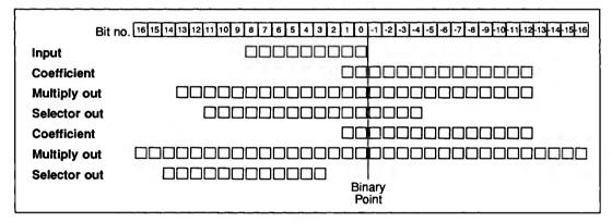
Figure 5.1 DCT internal number format
