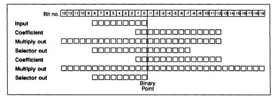
Figure 5.3 Filter and Transpose internal number format
