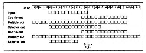
Figure 5.2 IDCT internal number format
