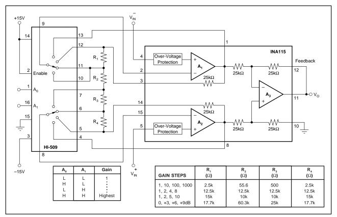
FIGURE 2. Switched-Gain Instrumentation Amplifier (minimum components).
