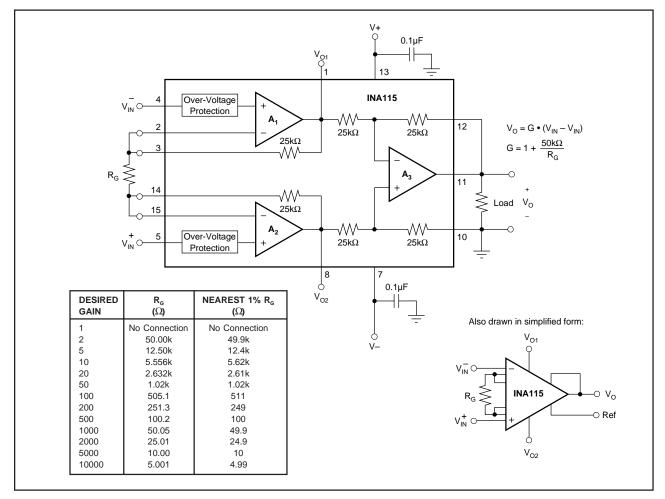
FIGURE 1. Basic Connections.
