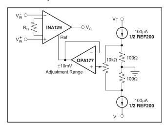
Figure 24. Optional Trimming of Output Offset Voltage
