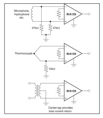
Figure 25. Providing an Input Common-Mode Current Path
