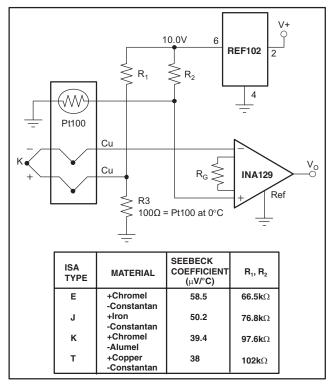
Figure 28. Thermocouple Amplifier With RTD Cold-Junction Compensation
