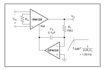
Figure 27. AC-Coupled Instrumentation Amplifier
