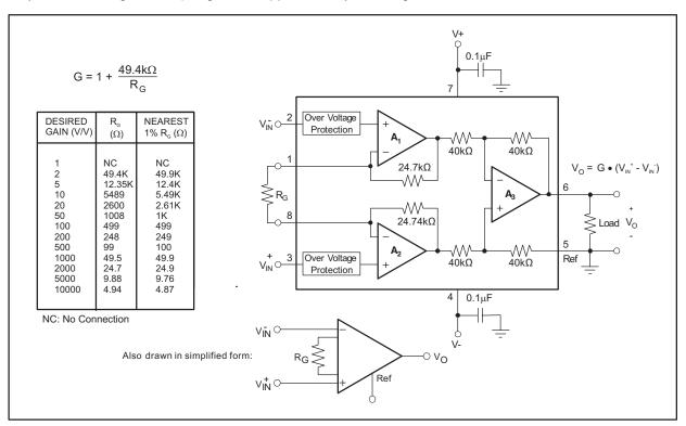
Figure 23. Basic Connections
