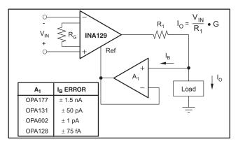
Figure 29. Differential Voltage to Current Converter
