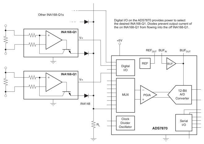
Figure 15. Multiplexed Measurement Using Logic Signal for Power
