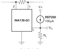
$\begin{aligned} & \text{Gain Set by R}_L \\ & \text{Output Offset} = (100\,\mu\text{A})(\text{R}_L) \\ & \text{(independent of V+)} \end{aligned}$
