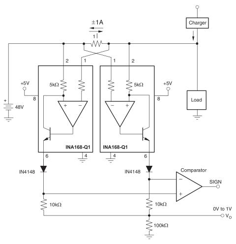
Figure 13. Bipolar Current Measurement
