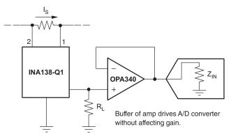
INA138-Q1  $f_{-3dB} = \frac{1}{2\pi R_L C_L}$   $R_L \qquad C_L$
