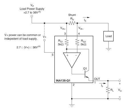
Figure 9. Basic Circuit Connections
