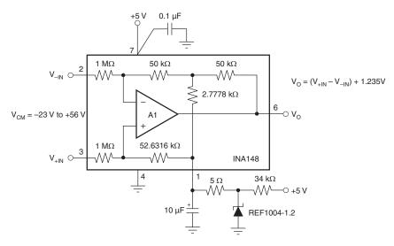
Figure 7. Single-Supply Differential Amplifier
