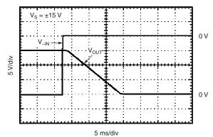
NON-INVERTING INPUT 50% OVERLOAD RECOVERY TIME
