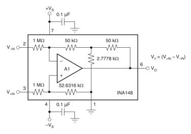
Figure 1. Basic Circuit Connections
