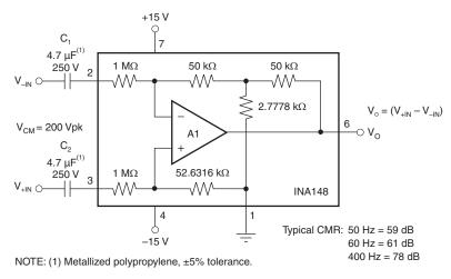
Figure 5. AC-Coupled Difference Amplifier
