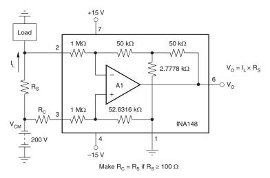
Figure 4. Shunt-Resistor Current Measurement Circuit
