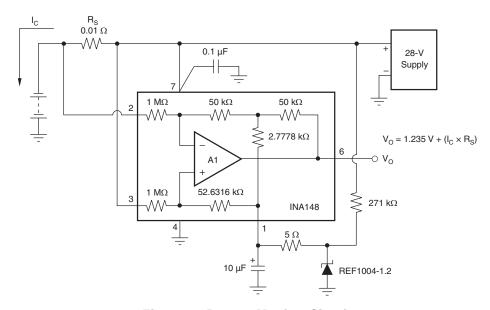
Figure 8. Battery Monitor Circuit
