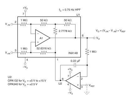
Figure 6. Quasi-AC-Coupled Differential Amplifier
