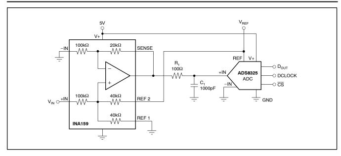
Figure 3. Typical Application Circuit Interfacing to Medium-Speed, Single-Supply ADCs
