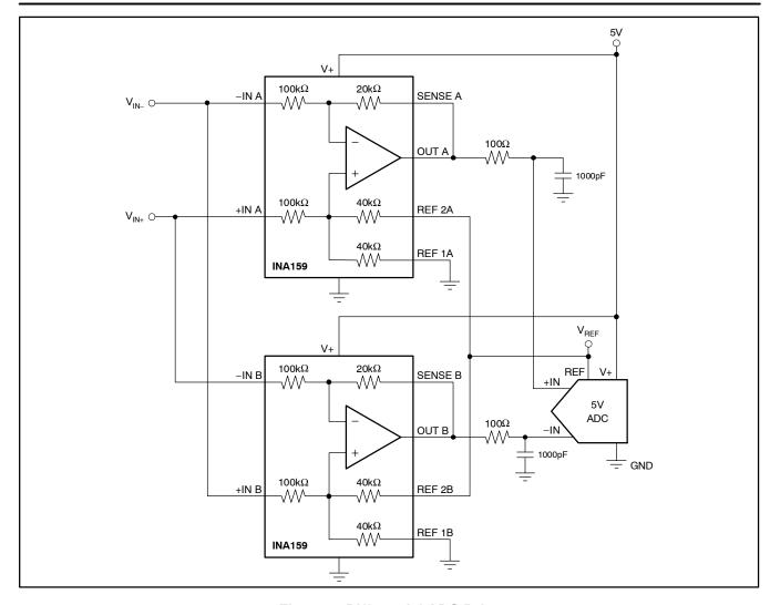
Figure 6. Differential ADC Drive
