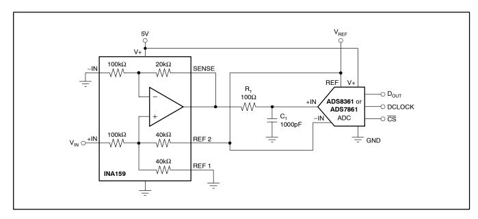
Figure 4. Typical Application Circuit Interfacing to Medium-Speed, Single-Supply ADCs with Pseudo-Differential Inputs (such as the ADS7861 and ADS8361)
