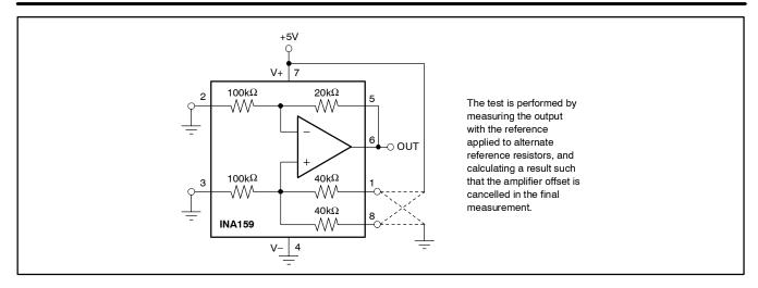
Figure 2. Test Circuit for Reference Divider Accuracy
