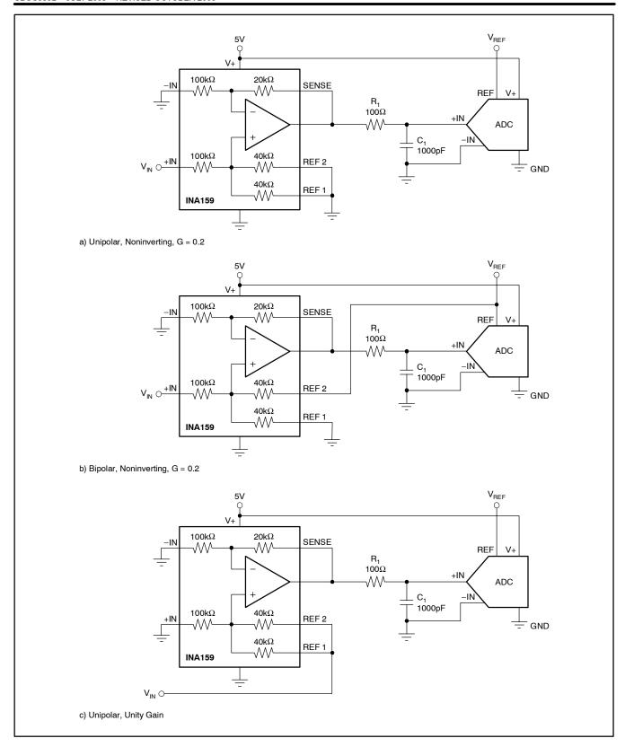
Figure 5. Basic INA159 Configurations
