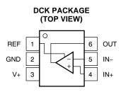
The INA213 and INA214 are voltage-output current-shunt monitors that can sense drops across shunts at common-mode voltages from -0.3 V to 26 V, independent of the supply voltage. The INA213 offers a fixed gain of 50 V/V, and the INA214 offers a fixed gain of 100 V/V. The low offset of the zero-drift architecture enables current sensing with maximum drops across the shunt as low as 10-mV full-scale.
