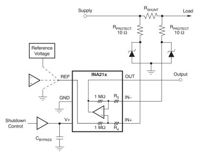
Figure 27. INA21x Transient Protection Using Dual Zener Diodes
