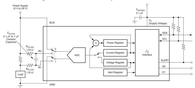
Figure 22. INA230 with Input Filtering
