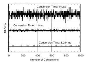
Figure 21. Noise vs Conversion Time
