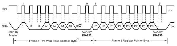
(1) The value of the slave address byte is determined by the settings of the A0 and A1 pins. Refer to Table 7.
