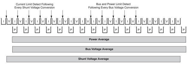
Figure 20. Power Calculation Scheme
