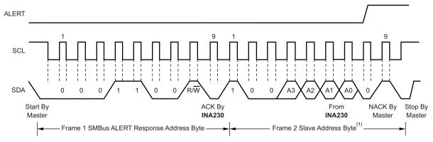
(1) The value of the slave address byte is determined by the settings of the A0 and A1 pins. Refer to Table 7.
