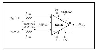
FIGURE 7. Sample Output Buffering Circuit.
