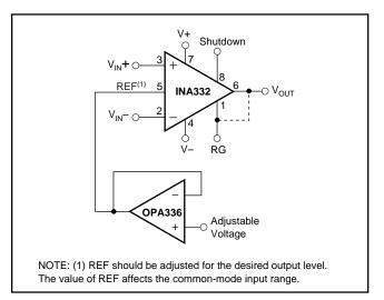
FIGURE 6. Optional Offset Trimming Voltage.
