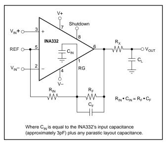
FIGURE 8. Feedback Capacitor Improves Dynamic Performance.
