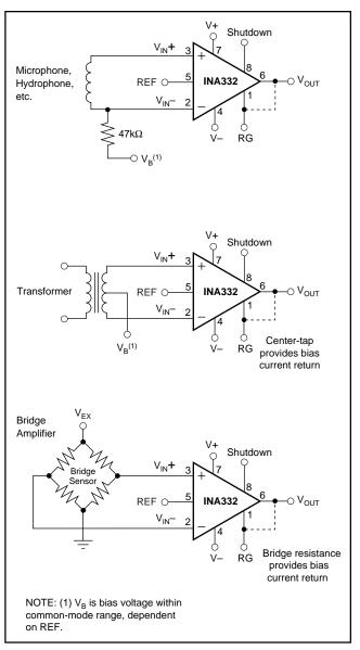
FIGURE 3. Providing an Input Common-Mode Path.
