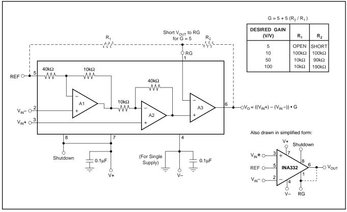
FIGURE 1. Basic Connections.
