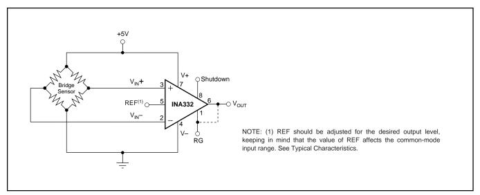
FIGURE 2. Single-Supply Bridge Amplifier.
