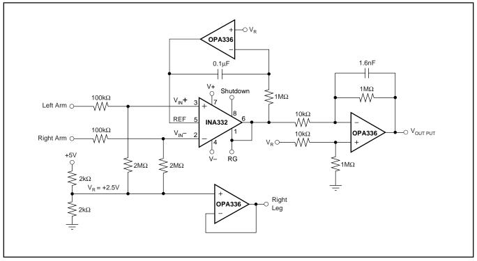
FIGURE 9. Simplified ECG Circuit for Medical Applications.
