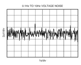
At T<sub>A</sub> = +25°C, V<sub>S</sub> = 5V, V<sub>CM</sub> = V<sub>S</sub>/2, R<sub>L</sub> = 10kΩ, and C<sub>L</sub> = 100pF, unless otherwise noted.
