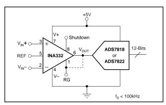
FIGURE 4. INA332 Directly Drives Capacitive-Input, High-Speed A/D Converter.
