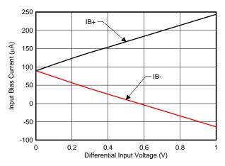
Figure 33. Input Bias Current vs Differential Input Voltage
