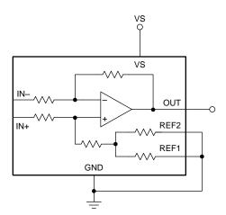
Figure 26. Ground Referenced Output
