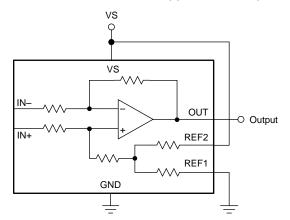
Figure 29. Midsupply Voltage Output
