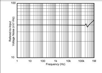
Figure 18. Input-Referred Voltage Noise vs Frequency
