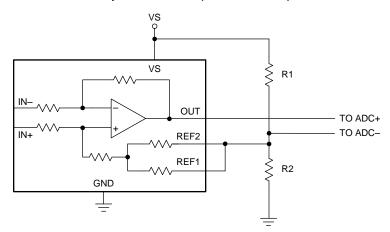
Figure 31. Setting the Reference Using a Resistor Divider
