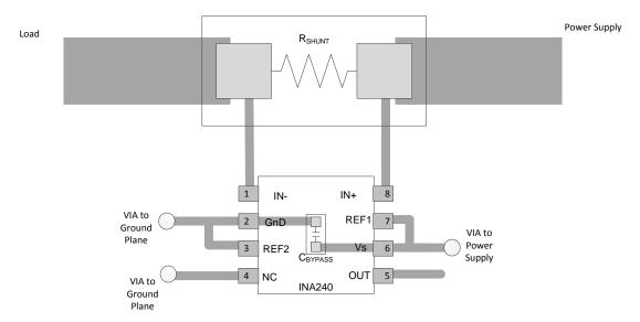
Figure 40. Recommended SOIC Package Layout
