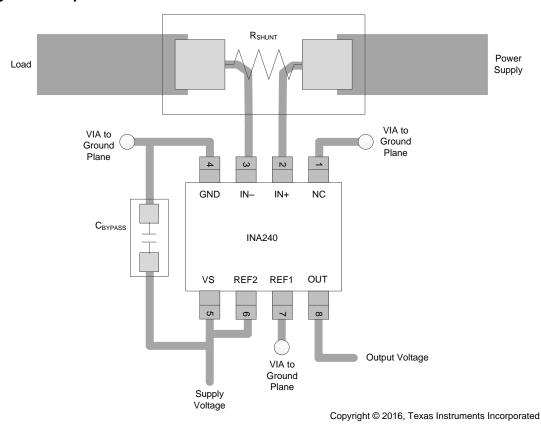
Figure 39. Recommended TSSOP Package Layout
