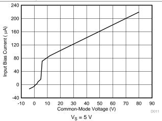
Figure 14. Input Bias Current vs Common-Mode Voltage
