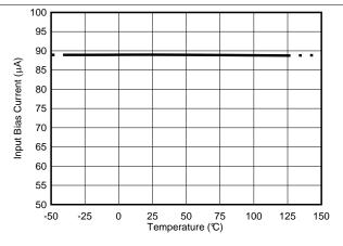
Figure 16. Input Bias Current vs Temperature
