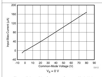
Figure 15. Input Bias Current vs Common-Mode Voltage
