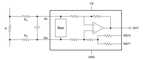
Figure 32. Filter at Input Pins
