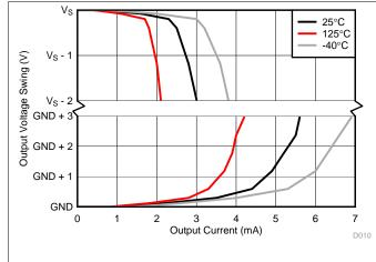
Figure 13. Output Voltage Swing vs Output Current
