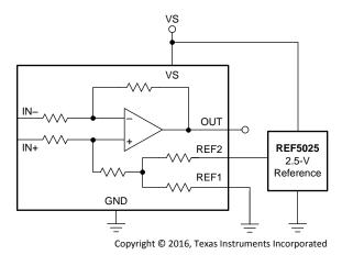
Figure 30. Mid-External Reference Output
