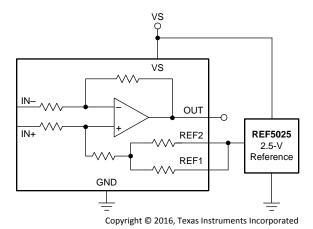
Figure 28. External Reference Output
