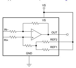
Figure 27. VS Referenced Output
