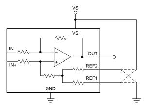
Figure 25. Test Circuit For Reference Divider Accuracy
