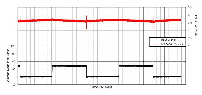
Figure 35. Inline Motor Current-Sense Input and Output Signals
