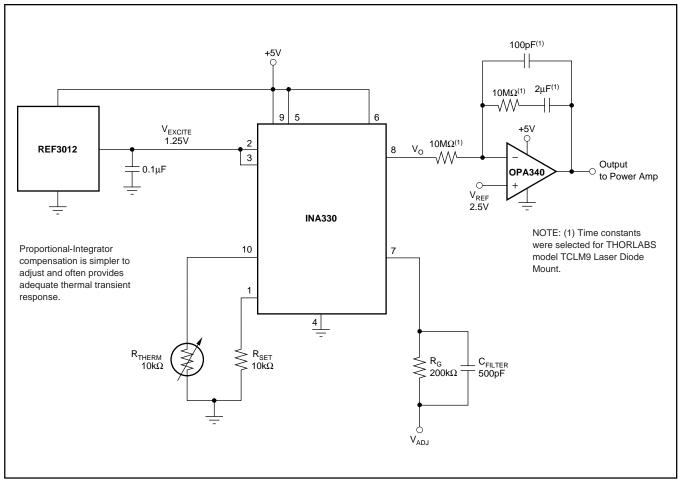
FIGURE 8. Simple PI Temperature Control Amplifier.
