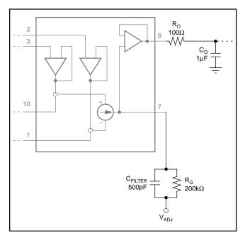
FIGURE 9. Required 1.6kHz (or lower) Filtering.
