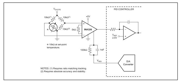
FIGURE 11. Traditional Bridge Circuit.
