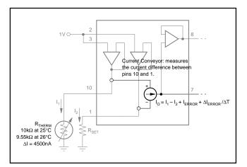
FIGURE 2. Current Conveyor Portion of the INA330.
