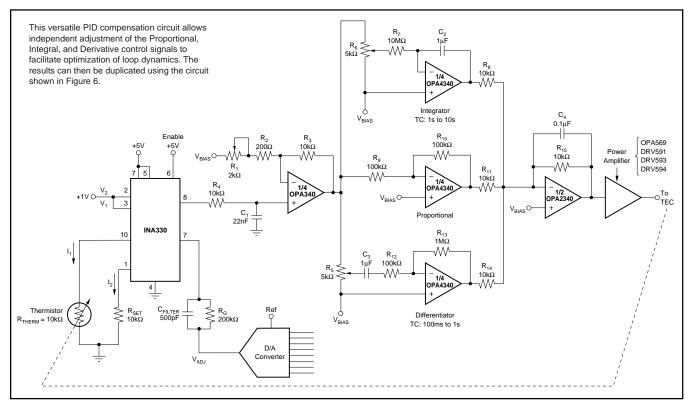
FIGURE 7. Diagnostic and Optimization PID Temperature Control Loop.
