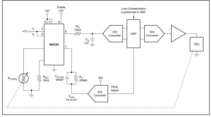
FIGURE 10. Digitally Compensated Loop.
