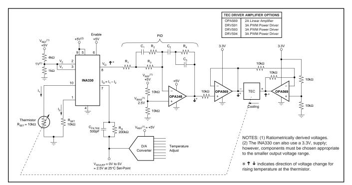
FIGURE 6. PID Temperature Control Loop.
