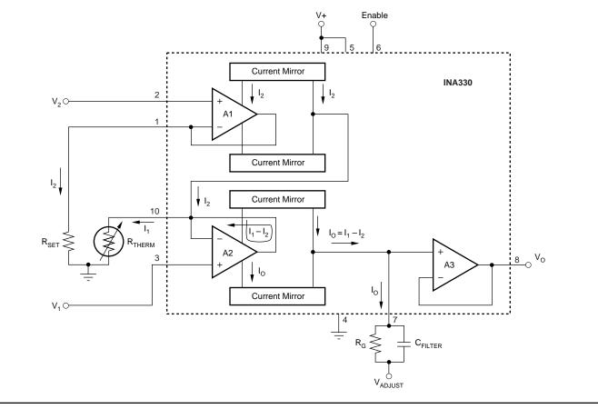
FIGURE 5. INA330 Simplified Schematic.
