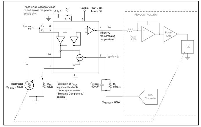
FIGURE 1. The INA330 In Simplified Temperature Control Loop.
