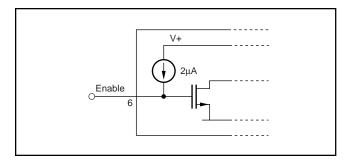
FIGURE 4. Enable Pin Model.
