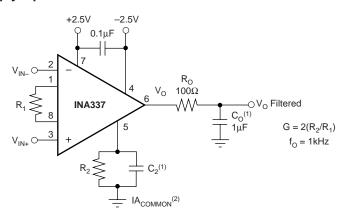
NOTES: (1)  $\rm C_2$  and  $\rm C_0$  combine to form a 2-pole response that is –3dB at 1kHz. Each individual pole is at 1.5kHz. (2) Output voltage is referenced to IA $_{\rm COMMON}$  (see text).
