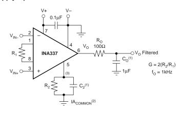
NOTES: (1)  $C_2$  and  $C_0$  combine to form a 2-pole response that is -3dB at 1kHz. Each individual pole is at 1.5kHz. (2) Output voltage is referenced to IA<sub>COMMON</sub> (see text). (3) Output pedestal required for measurement near zero (see Figure 6).
