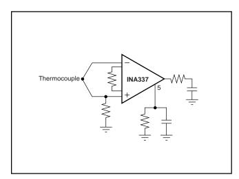
FIGURE 3. Providing Input Bias Current Return Path.
