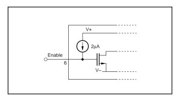
FIGURE 5. Enable Pin Model.
