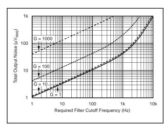
FIGURE 2. Total Output Noise vs Filter Cutoff Frequency.
