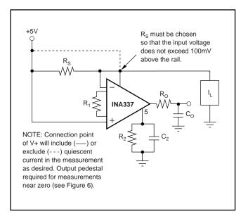
FIGURE 7. High-Side Shunt Measurement of Current Load.
