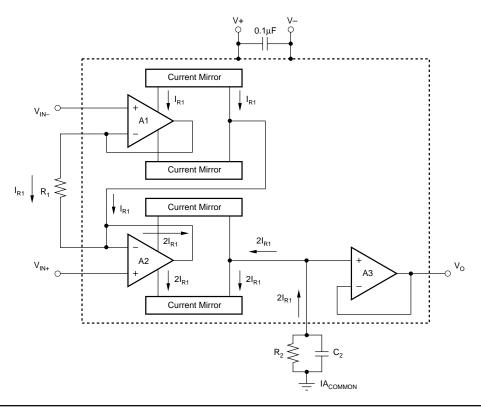
FIGURE 4. Simplified Circuit Diagram.
