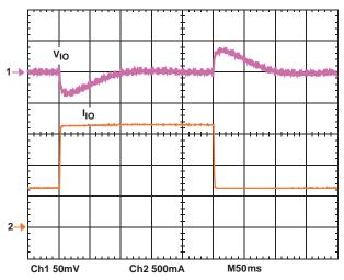
FIGURE 9. I/O CONVERTER LOAD TRANSIENT IN PWM MODE
