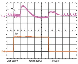
FIGURE 10. I/O CONVERTER LOAD TRANSIENT WITH MODE CHANGE
