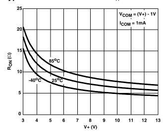
FIGURE 7. ON RESISTANCE vs SUPPLY VOLTAGE
