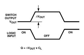
FIGURE 2A. MEASUREMENT POINTS
