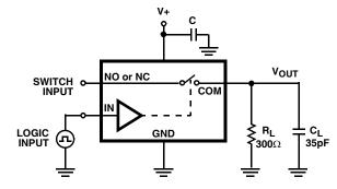
FIGURE 1B. TEST CIRCUIT
