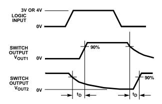
FIGURE 3A. MEASUREMENT POINTS (ISL5122 ONLY)
