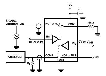
FIGURE 6. CROSSTALK TEST CIRCUIT
