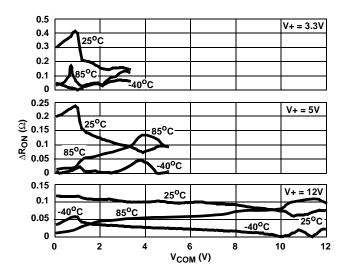
FIGURE 11. RON MATCH vs SWITCH VOLTAGE
