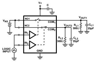
$C_L$  includes fixture and stray capacitance.
