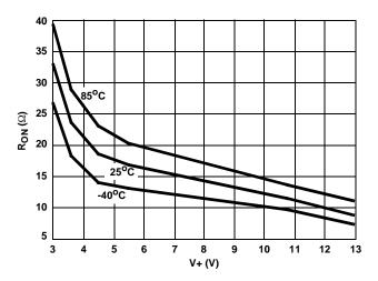
FIGURE 9. ON RESISTANCE vs SUPPLY VOLTAGE
