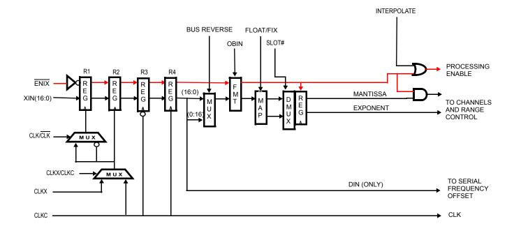
NOTE: To simplify the board routing, each of the four input data busses can be reversed, MSB for LSB (see IWA = 0\*00h, bit 4)
