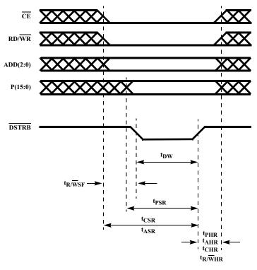
FIGURE 15. MICROPROCESSOR WRITE TIMING ( $\mu$ P mode = 1))
