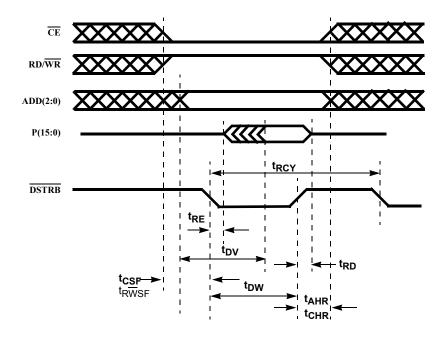
FIGURE 16. MICROPROCESSOR READ TIMING ( $\mu$ P mode = 1))
