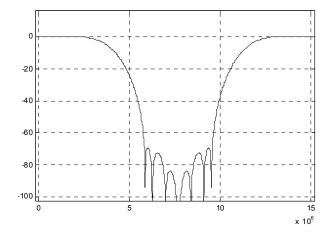
FIGURE 7A. INTERPOLATION HALF BAND RESPONSE
