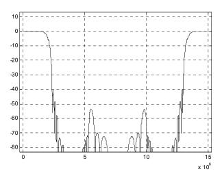
FIGURE 7E. FIR2 AND IHBF COMPOSITE RESPONSE
