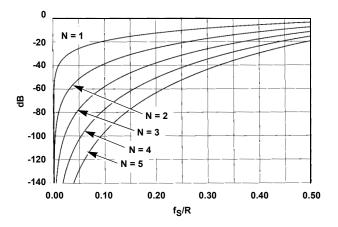
FIGURE 19A. CIC FIRST ALIAS LEVEL (N = # OF STAGES, R = DECIMATION FACTOR, fg/R = 1 is CIC OUTPUT RATE)
