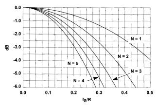
FIGURE 19. CIC PASSBAND ROLLOFF (N = # OF STAGES, R = DECIMATION FACTOR, fg/R = 1 is CIC OUTPUT RATE)
