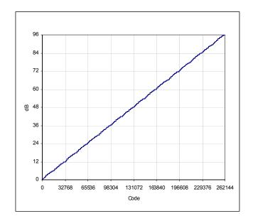
FIGURE 5A. ISL5416 AGC FORWARD GAIN RESPONSE
