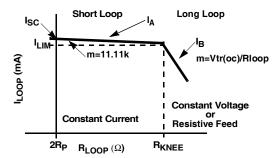
FIGURE 3. ILOOP vs. RLOOP LOAD CHARACTERISTIC
