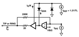
FIGURE 1. CURRENT LIMIT FUNCTIONAL DIAGRAM
