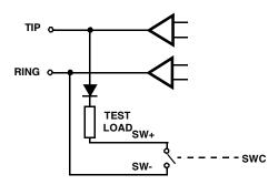
FIGURE 16. TEST LOAD SWITCHING
