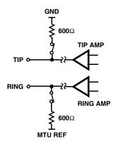
FIGURE 8. LPS 2-WIRE INTERFACE CIRCUIT DIAGRAM
