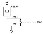
FIGURE 15. EXTERNAL RELAY SWITCHING
