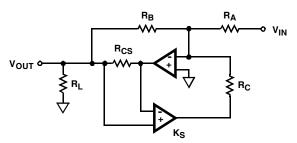
FIGURE 9. VOLTAGE FEED CURRENT SENSE DIAGRAM
