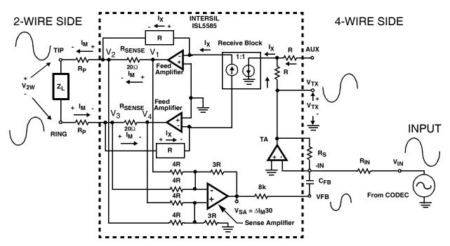
FIGURE 6. 4-WIRE TO 2-WIRE SIGNAL PHASE ACROSS THE ISL5585
