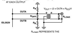
FIGURE 7. ALTERNATIVE OUTPUT LOADING
