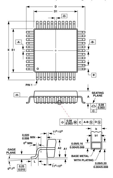
Q48.7x7A (JEDEC MS-026BBC ISSUE B) 48 LEAD THIN PLASTIC QUAD FLATPACK PACKAGE
