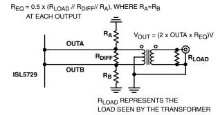
FIGURE 14. ALTERNATIVE OUTPUT LOADING
