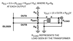
FIGURE 14. ALTERNATIVE OUTPUT LOADING
