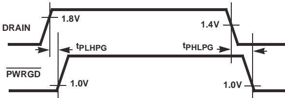
FIGURE 4A. DRAIN TO PWRGD TIMING (ISL6140)
