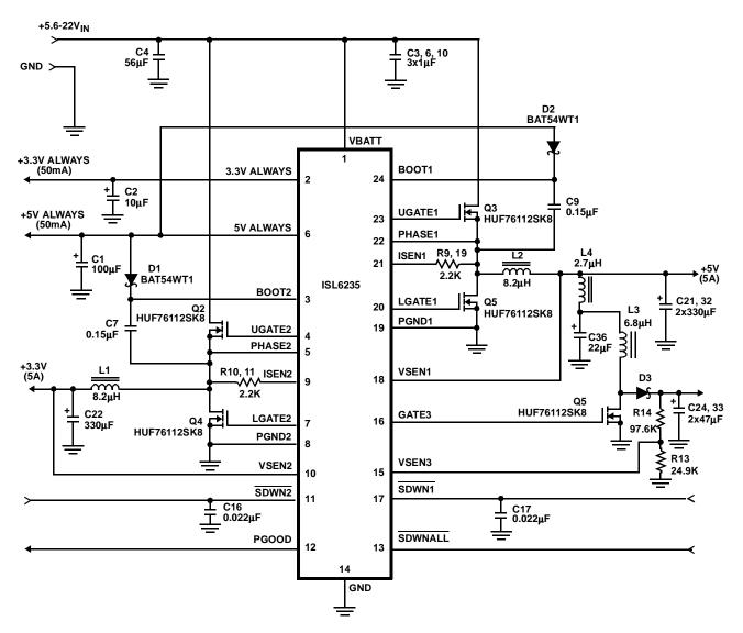
FIGURE 6. APPLICATIONS CIRCUIT
