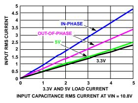
FIGURE 4. INPUT RMS CURRENT VS LOAD
