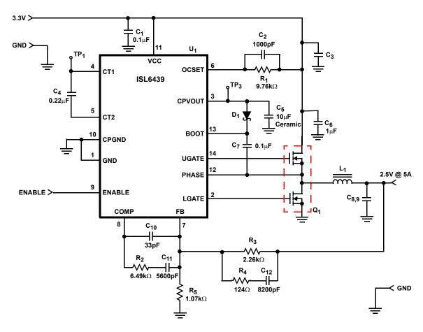
FIGURE 8. 3.3V to 2.5V 5A DC-DC CONVERTER
