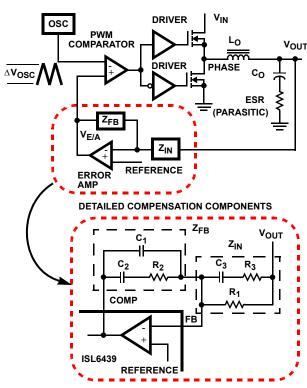
FIGURE 5. VOLTAGE-MODE BUCK CONVERTER COMPENSATION DESIGN
