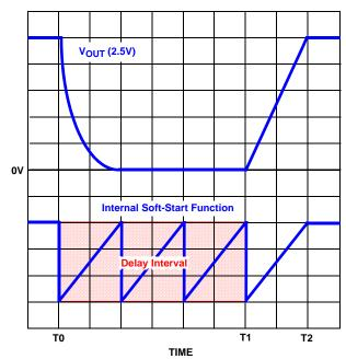
FIGURE 3. OVER CURRENT PROTECTION RESPONSE  $r_{DS(ON)}$  variations. To avoid overcurrent tripping in the normal operating load range, find the  $R_{OCSET}$  resistor from the equation above with:
