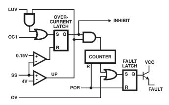
FIGURE 3. FAULT LOGIC - SIMPLIFIED SCHEMATIC
