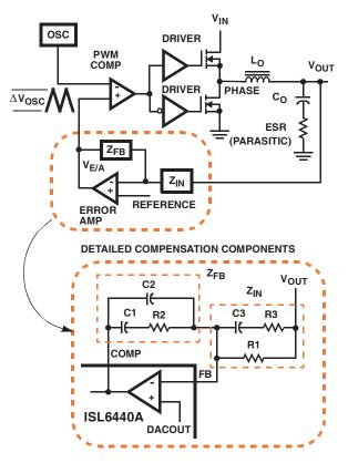
FIGURE 8. VOLTAGE-MODE BUCK CONVERTER COMPENSATION DESIGN
