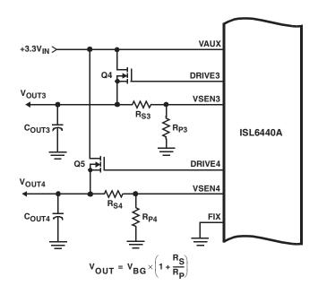
FIGURE 6. ADJUSTING THE OUTPUT VOLTAGE OF OUTPUTS 3 AND 4
