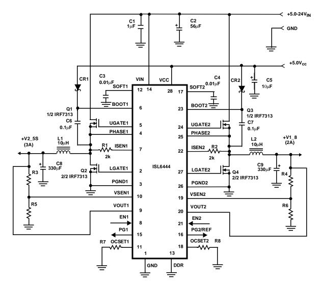
FIGURE 9. DUAL OUTPUT APPLICATION CIRCUIT FOR ONE-STEP CONVERSION
