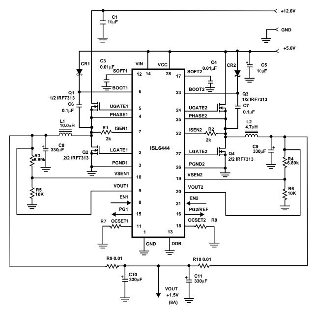
FIGURE 11. SINGLE-OUTPUT SPLIT INPUT POWER SUPPLY
