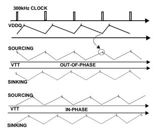
FIGURE 7. CHANNEL INTRFEARENCE Vin=7.5V...24V
