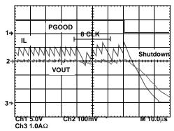
FIGURE 6. OVERCURRENT PROTECTION WAVEFORMS
