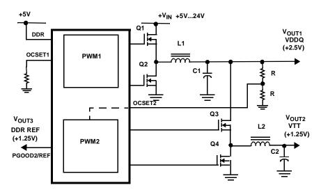
ISL6444 APPLICATION CIRCUIT FOR COMPLETE DDR MEMORY POWER SUPPLY
