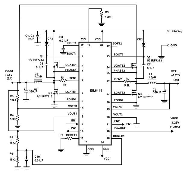
FIGURE 13. APPLICATION CIRCUIT FOR COMPLETE DDR MEMORY POWER SOLUTION WITH TWO-STEP CONVERSION
