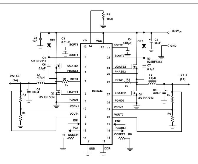
FIGURE 10. DUAL OUTPUT APPLICATION CIRCUIT FOR TWO-STEP CONVERSION
