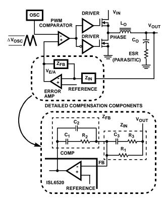
FIGURE 5. VOLTAGE-MODE BUCK CONVERTER COMPENSATION DESIGN
