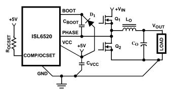
FIGURE 4. PRINTED CIRCUIT BOARD SMALL SIGNAL LAYOUT GUIDELINES
