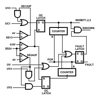
FIGURE 7. FAULT LOGIC - SIMPLIFIED SCHEMATIC
