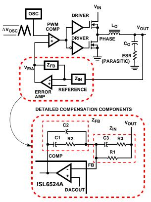
FIGURE 11. VOLTAGE-MODE BUCK CONVERTER COMPENSATION DESIGN
