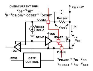
FIGURE 9. OVER-CURRENT DETECTION
