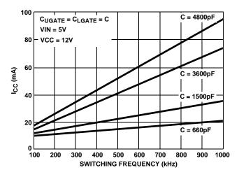
FIGURE 5. BIAS SUPPLY CURRENT vs FREQUENCY
