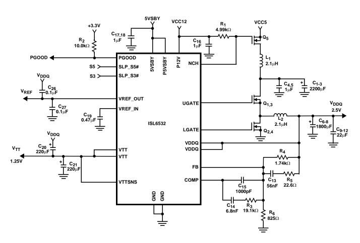
FIGURE 7. DDR SDRAM AND AGP VOLTAGE REGULATOR USING THE ISL6532
