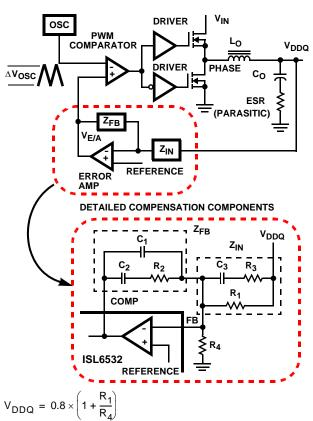
FIGURE 5. VOLTAGE-MODE BUCK CONVERTER
