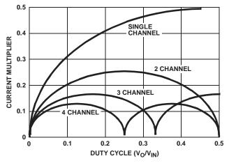
FIGURE 13. CURRENT MULTIPLIER vs DUTY CYCLE
