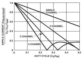
FIGURE 11. RIPPLE CURRENT vs DUTY CYCLE
