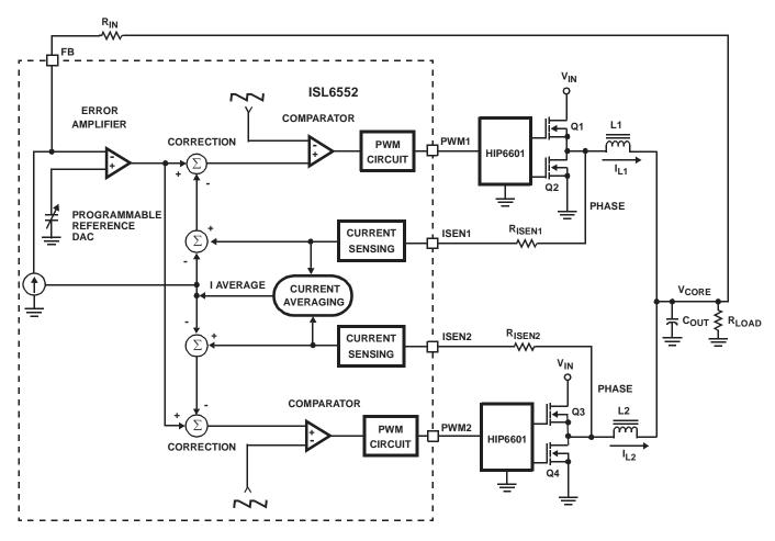
FIGURE 1. SIMPLIFIED BLOCK DIAGRAM OF THE ISL6552 VOLTAGE AND CURRENT CONTROL LOOPS FOR A TWO POWER CHANNEL REGULATOR
