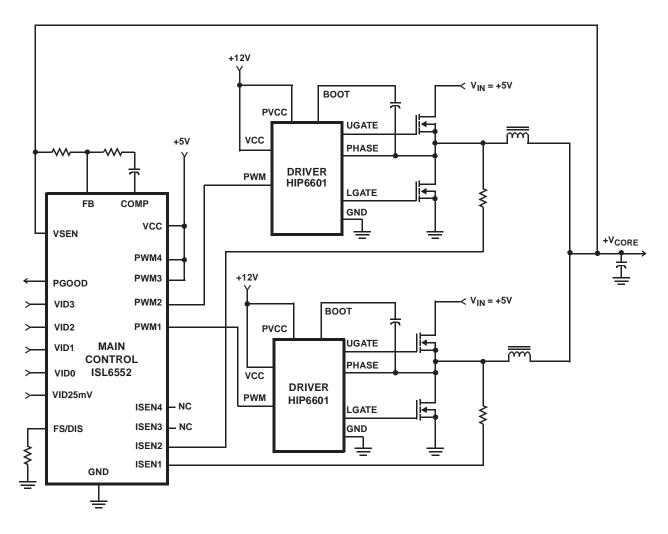
Typical Application - 4 Phase Converter Using HIP6602 Gate Drivers
