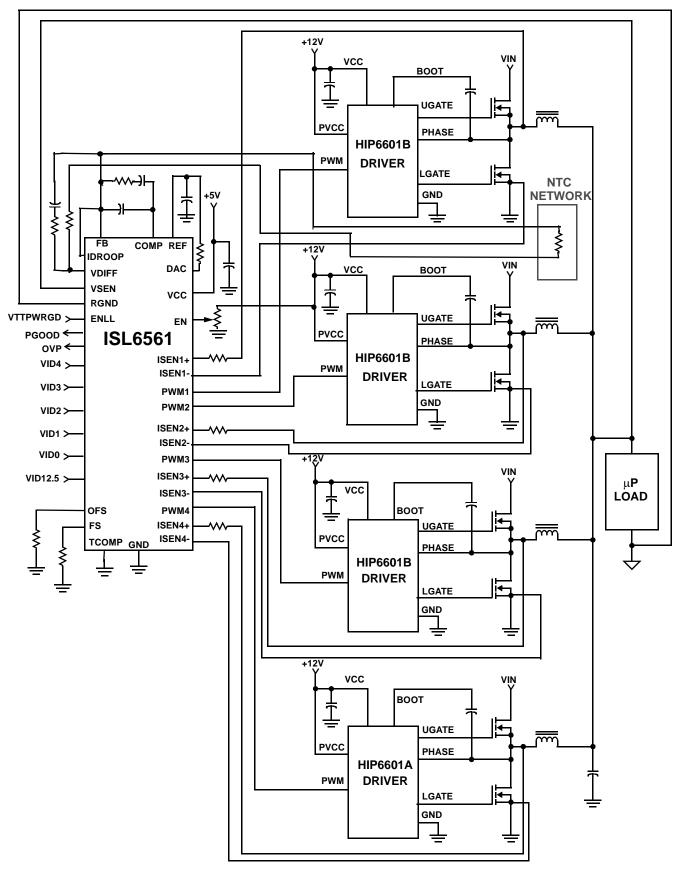
Typical Application - 4-Phase Buck Converter with Rds, On Sensing and External NTC
